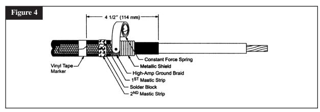
1.6 Wrap two half-lapped layers of vinyl tape around the mastic seal, constant force spring and exposed metallic shield. Do not cover cable semi-con.
