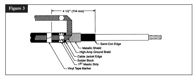
1.5 Wrap the ground strap around the metallic shield and secure with a constant force spring. Using the second strip of mastic, remove the liners and wrap mastic over the solder blocks and the first mastic strip. If the solder blocks overlap each other, mastic must be applied between the solder blocks.
