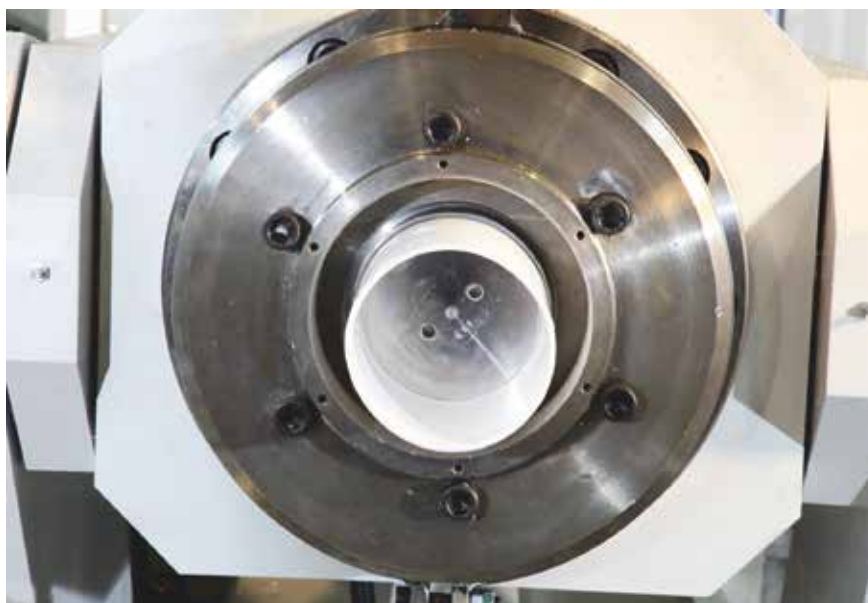
Fig. 1. Extruder head for the manufacture of a paste-extruded pipe made of PTFE
