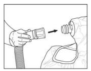
Inspect hood for tears, holes. Insert breathing tube into hood connection.
