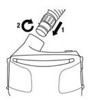
Insert breathing tube into PAPR air outlet.
