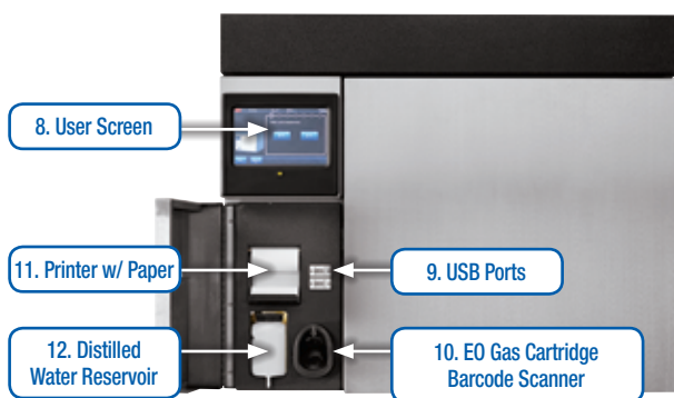
Figure 7. Front Panel, 3M™ Steri-Vac™ Sterilizer/Aerator GSX Series, Model GS5X
