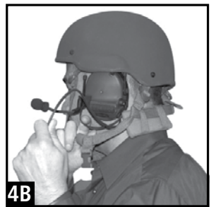
4B: Next, thread the down lead through the chinstrap.
