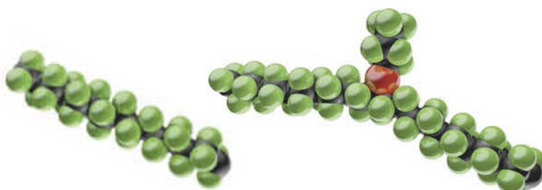
The molecular structure of PTFE (left) and modified PTFE (right): perfluoropropylvinyl ether (PPVE) is incorporated into the PTFE polymer chains, which simultaneously have a reduced molecular weight
