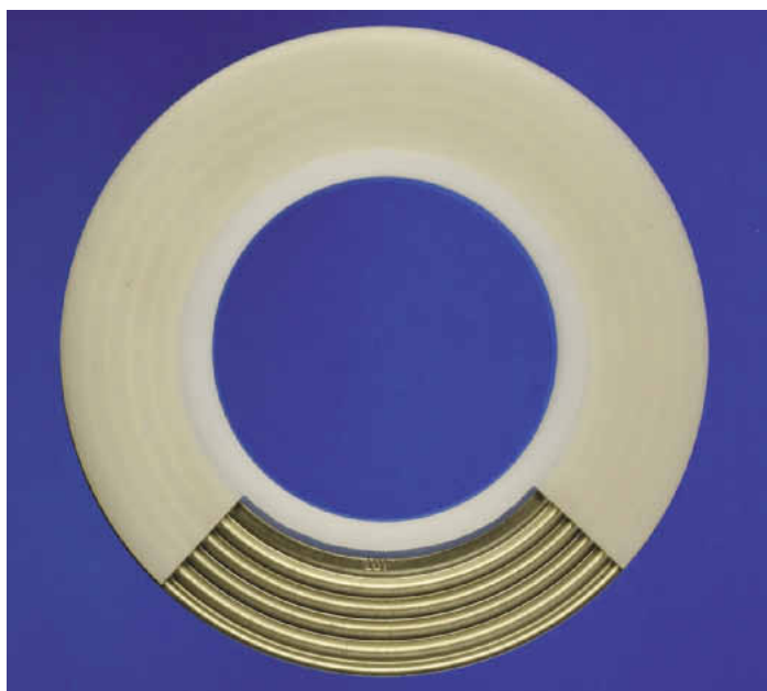
The PW-I gasket consists of a Dyneon TFM 1600 shell with an inner diffusion barrier and a stainless steel corrugated ring insert
